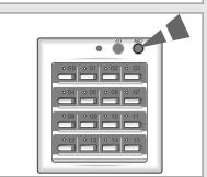
3 To turn off the all of air conditioners connected to the centralized controller, press the (All OFF) button.
